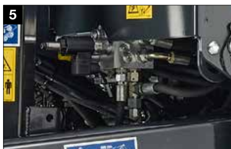
5 Pressdichteregelung POWER LOCK
