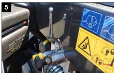
5 Pressdichteregelung POWER LOCK
